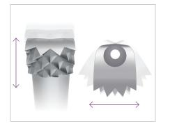
Couples longitudinal with torsional vibration for a 25,000x per second non-rotational motion that cuts bone without affecting soft tissue.
