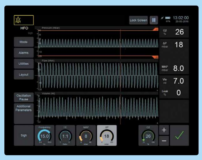
Switching to HFOV is a button-push away, and does not require any changes to the patient circuit. Parameter controls have changed to reflect the new mode. The 'Additional Parameters' button can display secondary controls for this mode. Selecting any parameter activates the + and - keys to adjust the parameter value.
