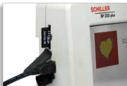
USB interface for calibrating the BP-200 plus and SD card for software update or research work
